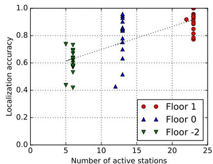
Figure 3. Localization accuracy on different floors of the Offices testbed (max training). Each point represents one test session.
