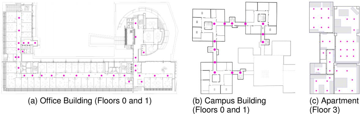
Figure 1. Testbed floorplans (color dots indicate the sampling locations — test points).
