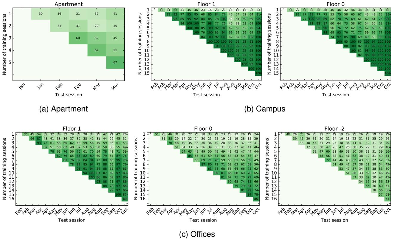
Figure 5. Positioning performance over time, with incremental training. Numbers in the cells are localization accuracy in percents. Random-guess levels are 3% for Apartment, 8% for Campus, and 3%, 3%, and 6% for floors 1, 0 and -2 of the Offices tested.
