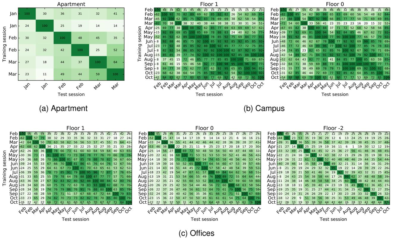
Figure 4. Positioning performance over time, with pairwise evaluation. Numbers in the cells are localization accuracy in percents. Random-guess levels are 3% for Apartment, 8% for Campus, and 3%, 3%, and 6% for floors 1, 0 and -2 of the Offices testbed.
